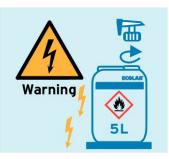
7. Attention: Carefully read the safety instructions below. Secure grounding before handling/opening canisters. Open 5 L canister for the refill procedure only and screw on filling tap. Place the canister on its side at an elevated position with the valve in the lowest position.
